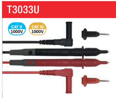
T3033U Probe Length: 119mm/ \phi 9\text{mm} Length: 800mm Tip: \phi 2\text{mm} Plug: \phi 4.5\text{mm} Wire: UL 1803/20AWG MAX 10A
