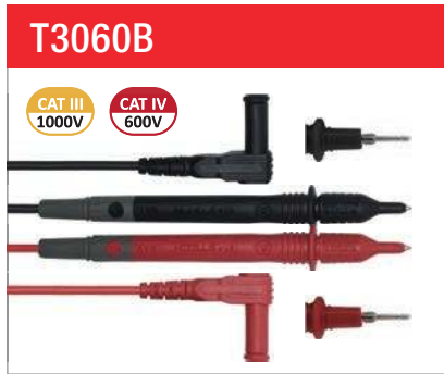
T3060B Probe Length: 132mm/ \phi 10\text{mm} Right Angle Type, M4 screw Length: 1500mm Tip: \phi 2\text{mm} Plug: \phi 4.5\text{mm} Wire: UL 1803/18AWG MAX 10A
