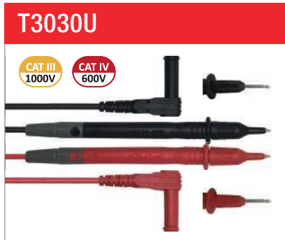
T3030U Probe Length: 143mm/ \phi 10\text{mm} Length: 1000mm Tip: \phi 2\text{mm} Plug: \phi 4.5\text{mm} Wire: UL 1803/18AWG MAX 10A
