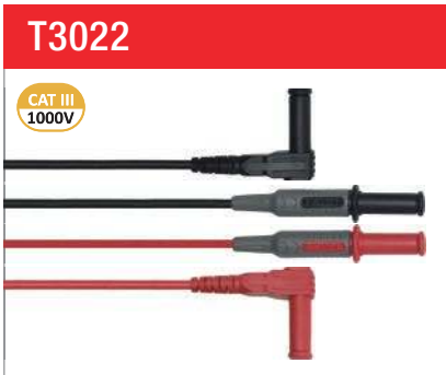
T3022 Straight Type & Right Angle Type Length: 1000mm Plug: \phi 4.5\text{mm} Wire: UL 1803/18AWG MAX 10A
