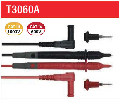
T3060A Probe Length: 132mm/ \phi 10\text{mm} Right Angle Type, M4 screw Length: 1000mm Tip: \phi 2\text{mm} Plug: \phi 4.5\text{mm} Wire: UL 1803/18AWG MAX 10A
